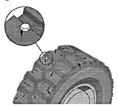
Check all wheel lug nuts or bolts to be sure none are loose or missing. Have missing bolts or lug nuts replaced and tightened to the the correct torque before operating truck. Torque to 100-120 lbf ft [135,6 - 162,7 N•m].
