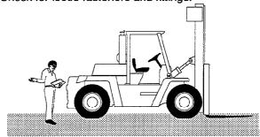
Check to be sure all capacity, safety and warning plates and decals are attached and legible.
