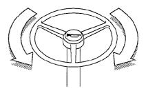
Check the operation of the neutral start switch by placing direction control lever inforward or reverse and turning key switch to START position. Starter must not engage until direction control lever is moved to NEUTRAL position.
