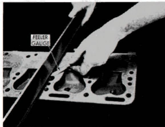
Figure 17 — Checking cylinder head flatness crosswise.
