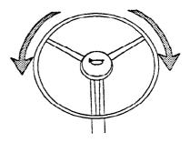
Return direction control to NEUTRAL and apply parking brake. Steer pump should stop.
