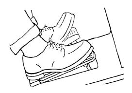
Retest service brake operation by applying and releasing the brakes several times while driving the truck. 1) Check for firm pedal pressure, quick pedal return, full stopping without pulling to one side, and for brake fading (must use more pedal effort each time to stop the truck). 2) Check for changes in pedal pressure. 3) Listen for brake squeal and other abnormal noise.
