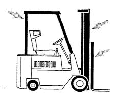
Check the overhead guard for damage. Be sure that it is properly positioned and all mounting fasteners are in place and tight.
