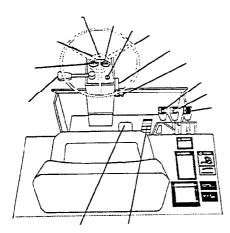
Check function of the parking brake mechanism. Release, then apply the parking brake with the lever. When correctly adjusted, the lever should snap-lock into the over-center applied position without having to use excessive force. If the lever binds or does not operate freely, apply lubricant to the linkage at pivot and sliding points.
