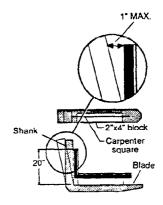
If the fork blades are obviously bent or damaged, have them inspected by a trained maintenance person.
