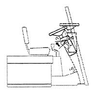
Check the service brake system. Push the brake pedal fully down and hold. The brakes should be applied before the pedal reaches the floorplate. Check for a feeling of solid resistance when the pedal stops. The pedal must feel firm and not move down farther after it stops. If the pedal continues to creep downwards, report the failure. DO NOT OPERATE THE TRUCK UNTIL THE BRAKES ARE REPAIRED.
