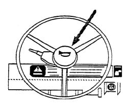
Press the horn button to check horn function. If the horn or any other part does not operate, report the failure and have it repaired before the truck is put back into operation.
