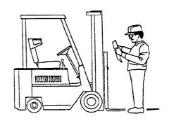
Check to be sure all capacity, safety, and warning plates or decals are attached and legible.
