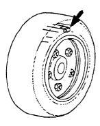
Check all wheel lug nuts or bolts to be sure none are loose or missing.
