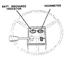
Check battery discharge indicator. The indicator should register in the green area when key switch is ON. Also, check function of battery discharge indicator when making a battery load test, below.
