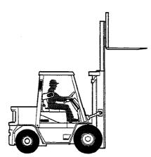
If the maximum fork height is not reached, this indicates there is an inadequate (low) oil level in the hydraulic sump tank or severe binding within the upright.
