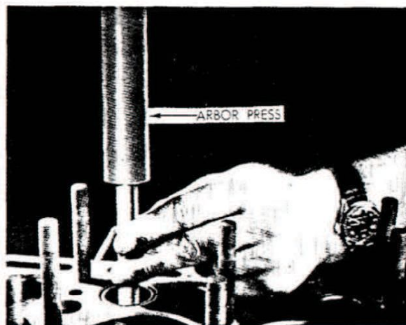
Figure 20 — Removing valve guides
