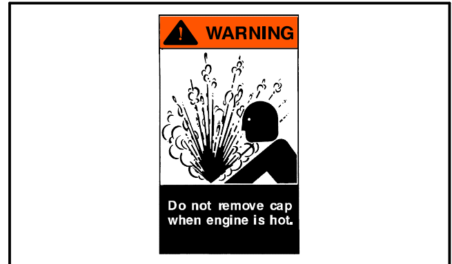
Figure 5 Allow engine to cool before removing the radiator cap.
