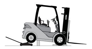
Put an equal amount of blocks under each side of the truck to provide a level working position.
