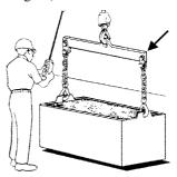
• Make sure that the chains and safety hooks are checked and offer a sufficient load carrying capacity. Never use chains fixed to a centre ring. These chains will pull the compartment walls to the inside, thus damaging the battery cells.
