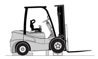
When maintenance work is completed, lower the truck to the floor by reversing the lifting procedure. Check to be sure no tools or equipment are under the truck or wheels.
