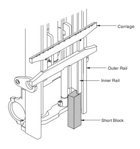
7. Reverse the procedure to remove blocking.
